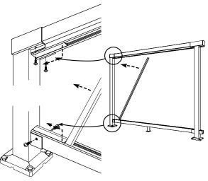
Remove the temporary post to install the last few pickets and spacers. Cut the last spacers flush with the ends of the rails. NOTE: to ensure equal picket spacing at each post, cut the first and the last spacers in the hand and base rails to equal lengths.
