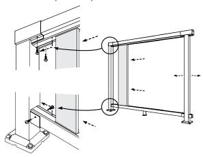
Insert the rails into the second post. Postion and fasten the second post in place - ensure that the post is plumb. Secure the rails to the second post with self-drilling screws. Repeat Steps 1-4 for each remaining section.
