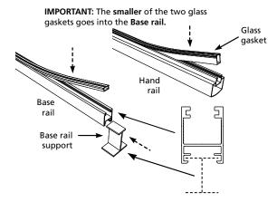
Insert the rails into the posts. Postion and fasten the second post in place - ensure that the post is plumb. Secure the rails to the posts with self-drilling screws. (Refer to Step 4 on Page 5.)
