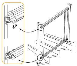
Place a picket into both rails near the bottom post - ensure that the picket is plumb and 4" or less from the post. Starting from the bottom post, measure and cut the **end spacers** then remove the picket (Fig. 1).
