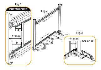
**PRO TIP:** To ensure equal spacing at each post, cut the first and last spacers in the hand and base rails to a length that ensures equal spacing between the end pickets and the posts.
