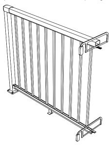
Insert the rails into the second post. Postion and fasten the second post in place - ensure that the post is plumb. Secure the rails to the second post with self-drilling screws. Repeat Steps 1-4 for each remaining section.
