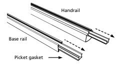
Cut the glass gaskets the same length as the rails and drill 1/8" holes into the base rail glass gasket for water drainage. Press the glass gaskets into the rails and install the base rail support into the bottom channel of the base rail.
