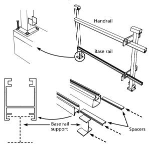
Insert the rails into the first post and secure these rails to this post with self-drilling screws. Use the second post as temporary support - do NOT secure the rails to the second post yet. Slide the first spacer in each rail against the first post. Insert a picket into the base rail and swing the top of the picket into the handrail as shown below. Repeat to complete the section.
