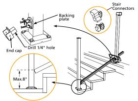
Cut the handrail to the same length as the base rail and fit the SCs onto the handrail. Use two **stair pickets** to position the handrail. Mark the locations of the SCs on the posts. Remove the handrail from position and the SCs from the handrail. Drill 7/32" pilot holes into the posts and use the flat head screws to attach the SCs to the posts. Temporarily move the bottom post to place the hand and base rails into the SCs. Secure the SCs to the rails at the bottom post only.
