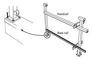
Remove the plastic picket gaskets from both rails.
