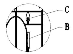
PLEASE USE ON/OFF TYPE"B" BULB MAX 40-WATT OR CFL BULB MAX 13-WATT OR LED BULB MAX 9-WATT
