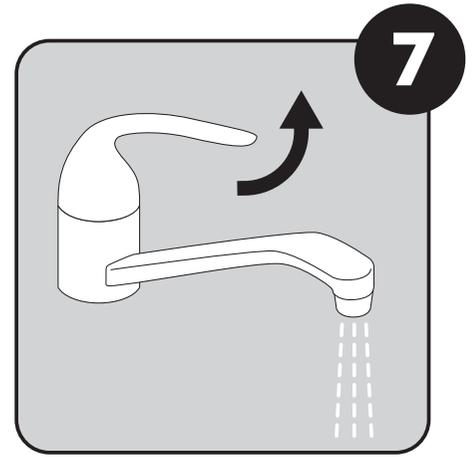
Turn on the cold water faucet and let it flush the new system for up to 5 minutes.
