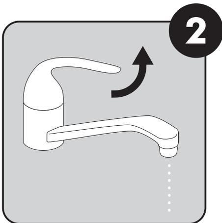
Turn the faucet handle to the **ON** position of cold water side to release the remaining water and relief the built-up pressure inside the system.
