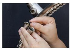
To attach the hose, begin by inserting a rubber washer into one end.
