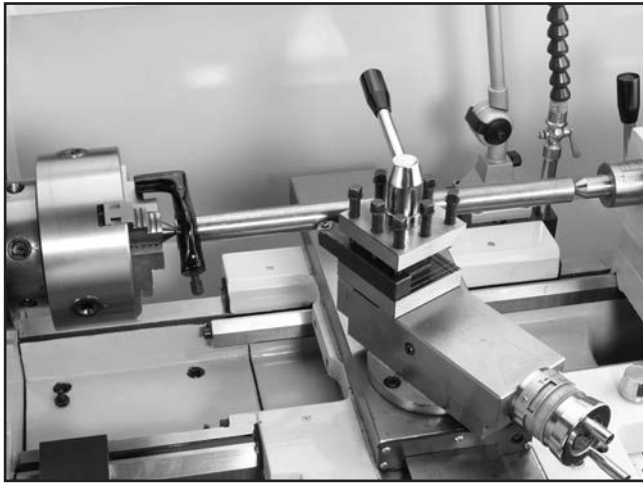
Figure 40. Example of stock mounted between the centers.
