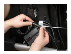
Plug the loose battery backup module into the extra lead on the sync cable.
