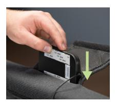
Move to the head of the base. Until the Sleeptracker sensors and insert them, white tape side towards you to ensure that the sensor is face-up, into the pockets at the head of each base. Be sure to insert all the way into the pocket. Secure with the Velcro straps.
