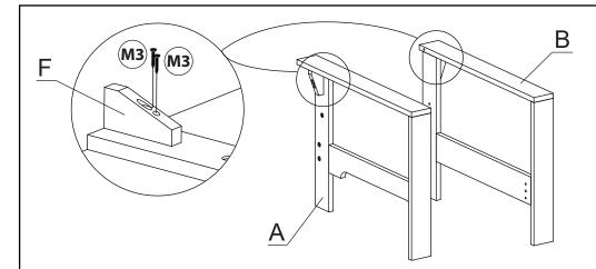
Step 1: Fix armrest supporting to the corner of leg frame as shown then secure using screw (M3). Fully tighten using screw driver
