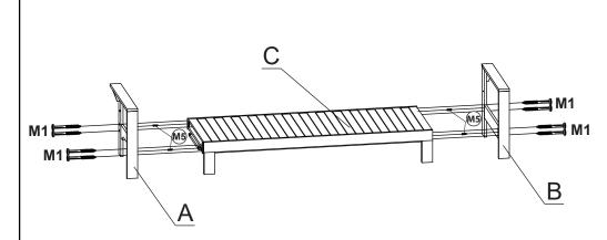
Step 3: insert Wooden dowel (M5) into the hole in seat (C) then attach the left leg frame (A) to Seat use screw (M1). Tighten using Allen Key (M6). Repeat for the right leg frame (B).Do not fully tighten Screw until all are installed.
