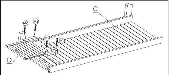
Step 2: Fix sliding tray to wooden bracket of seat as shown then Tighten using screw (M2) & Allen key (M6)
