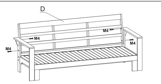
Step 4: Fix the backrest (D) to assembled frame then secure using Bolts (M4) & tighen with Allen key (M6)
