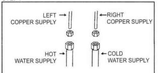
Carefully bend the copper supplies to meet the supply lines. Use the palms of your hands to bend, so as to avoid kinking.
