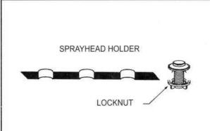
Separate locknut from sprayhead holder and insert sprayhead holder through sink. Reassemble and tighten locknut.
