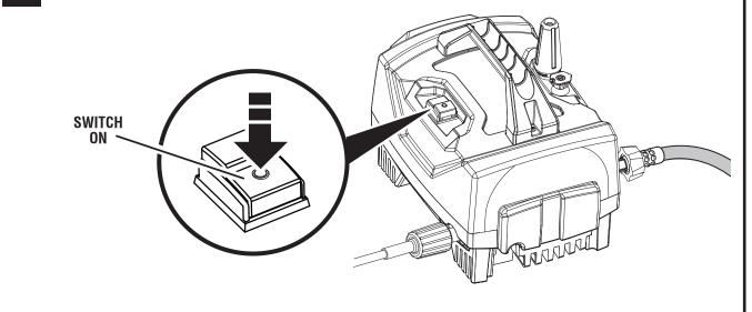
3 When finished, press switch OFF to stop the motor (see page 10).
