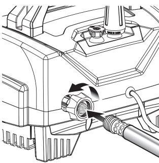
Completely uncoil garden hose or remove completely from reel to prevent kinks.
