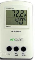
Combination digital hygrometer and thermometer measures humidity and temperature. Displays Fahrenheit or Celsius.
