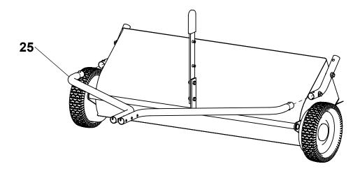
Install hardware through front two holes of Long Hitch Tubes as shown. Hold Adjustment Lever in position and install third bolt as shown. Pin Adjustment Lever to Handle.
