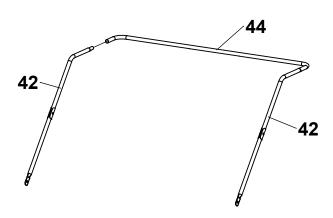
Place top frame assembly into Hopper Bag.
