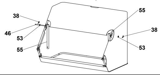
Hold Hopper Bag open and carefully insert Tension Rods into holes in Rear Frame Tubes.
