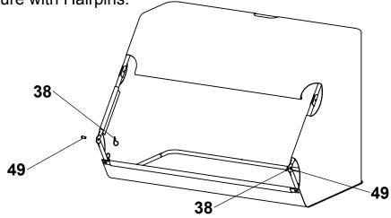
Slide Pivot Rod through Top Frame Tube and Connecting Tube, then through pocket of Hopper Bag, then through Connecting Tube and Top Frame Tube. Secure both ends with Washer and Hairpin.
