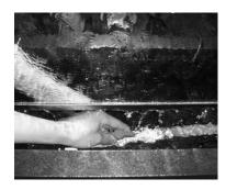
If the problem persists, please open the top cover without removing and while using the towel provided, clean the stainless steel barrier back & forth until the desired flow effect is achieved
