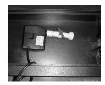
Thread and feed the pump cord through the opening provided in the reservoir. Pull the pump cord through the opening leaving approximately 12 inches of the cord inside the reservoir. DO NOT plug the pump into your local power supply.
