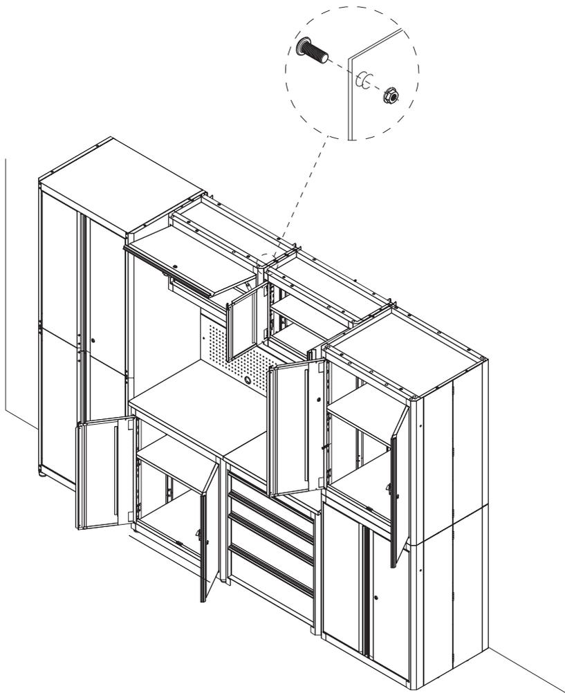
Hide holes on the exterior ends of the units with the supplied end covers, if necessary.
