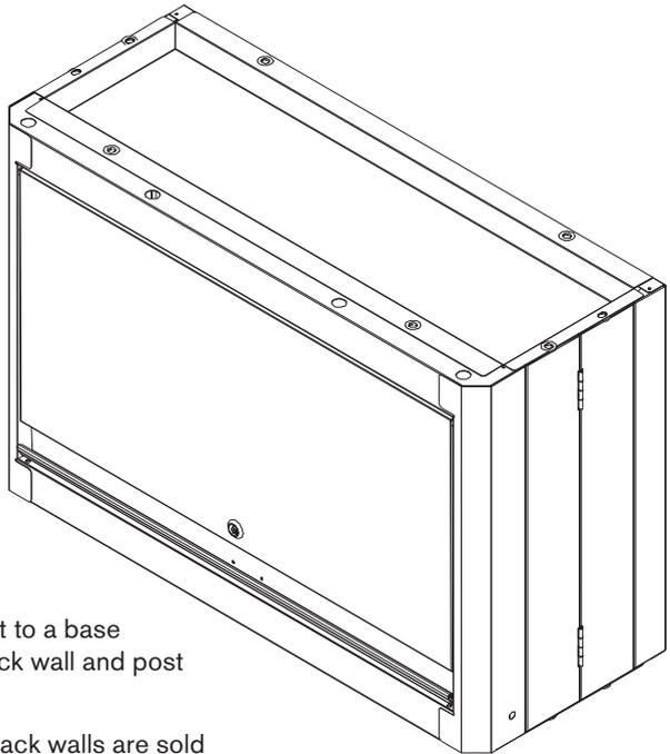
You can attach this wall cabinet to a base cabinet using the pegboard back wall and post combination.
