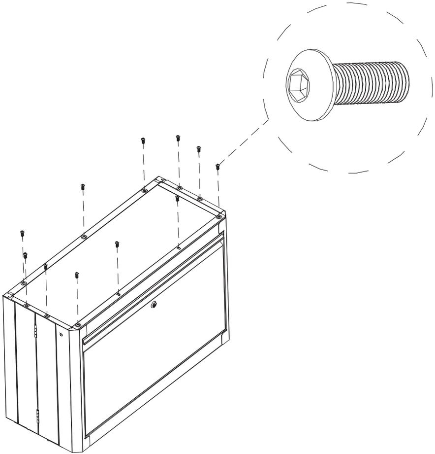
Turn the cabinet back to the upright position. Attach the top panel using eight M6 x 16 hex socket head screws.
