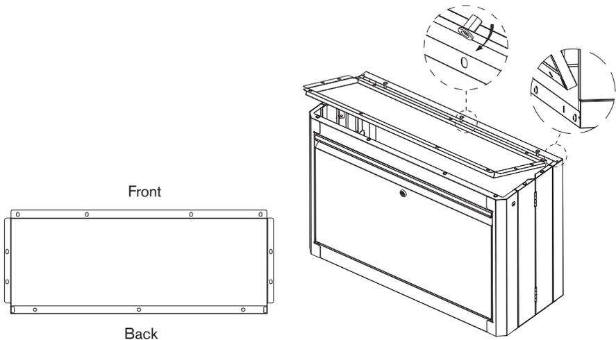
Attach the bottom panel using eleven M6 x 16 hex socket head screws.
