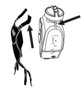
**3.** Pass end of the strap back through the buckle twice to secure in place and repeat on the other side.
