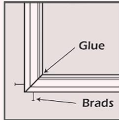
Most moldings are installed with a 90 degree angle joint. Cut 2 pieces of molding with a 45 degree angle each piece and together they make 90-degree angle. Use WPB Cement to glue the ends of the boards. On both sides place fasteners 2" from the end.
