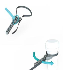
Turn wrench to the right/counterclockwise to tighten
