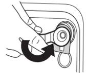
Hold the shipping bolt with your hand and pull it through the wide section of the hole. Repeat for each shipping bolt.
