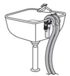
The drain hose must be placed at a height between 23.6 in (60cm) and 35.4 in (90cm).
