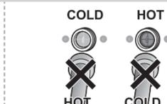
For proper operation, make sure both Hot & Cold hoses from faucets are connected to the corresponding Hot / Cold water inlets on the washer.
