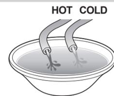
Run water in a bowl or basin to get rid of any debris inside hose. Check for HOT and Cold water supply.
