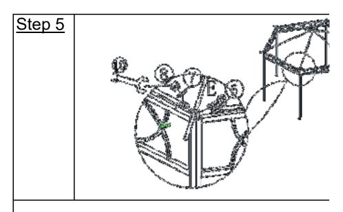
Attach Top Tubes(E) to Leg Tubes(A) using Bolts(6), Wash Spanners(10).
