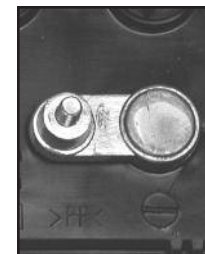
NEGATIVE POST HAS SMALLER DIAMETER
