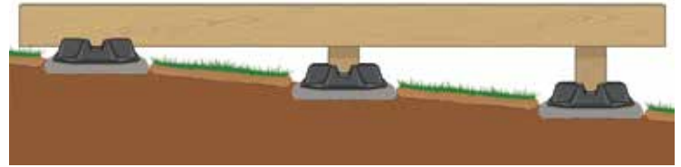
Use BLOCK on variable-height decks with posts and beams at various heights
