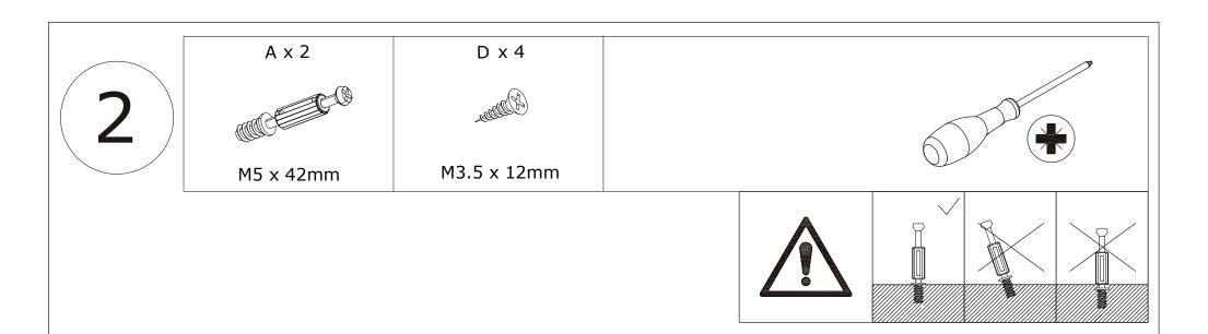
Fix No.13 slide rail to No.4 plate with screw(D) as shown. Insert quickfit screw(A) into corresponding holes in No.4 plate with a screwdriver as shown.
