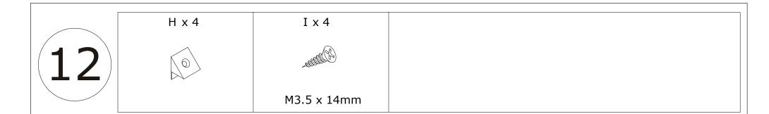
Reinforce back plate using part(H) and screw(I) as shown.
