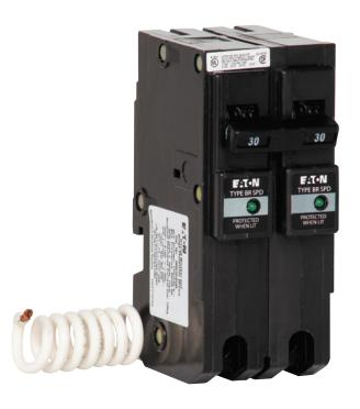
The BR surge breaker is designed to provide complete home surge protection for sensitive electronics and appliances from the damaging effects of surges. In addition to surge protection, the BR surge breaker is a functional 2-pole thermal magnetic breaker providing protection for overloads and short circuits.
