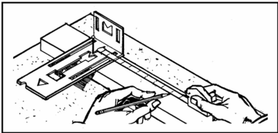
A small slot in the blade will hold the end of a tape measure, to pull room dimensions and stud layouts.
