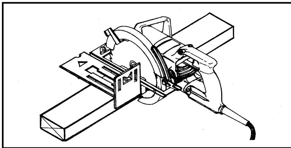
A saw guide for making square cuts with a circular saw.
