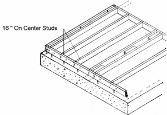
After marking top and sole plates, separate the plates and line up and nail studs as marked on plates.
