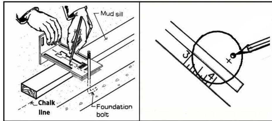
Transfer the anchor bolt locations to sill plate by placing the half moon shape
