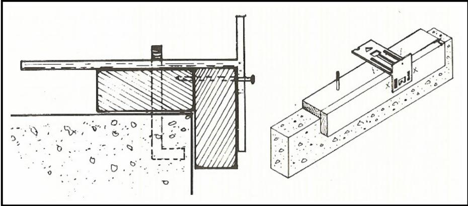
After drilling holes in sole plate, top and sole plate marked at the same time by placing sole plate over the foundation bolt then tacking the top plate on the side of the slab.
