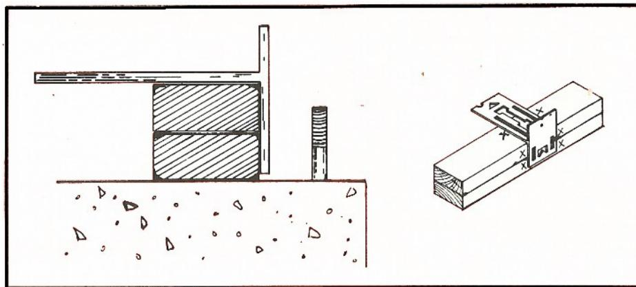
After stacking top and sole plates mark stud locations, middle partition and corner walls.
