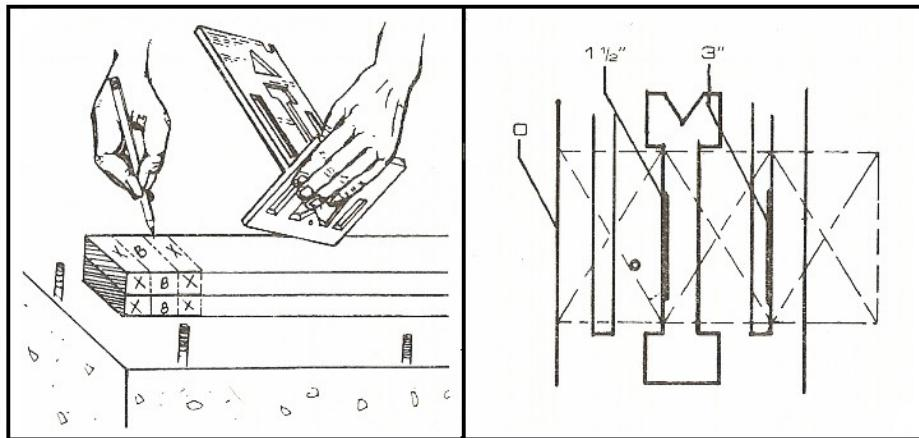
Three stud corners are easily layed out by placing the Lt on the corner of the top and sole plates and then mark as shown.
