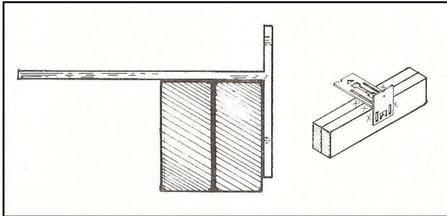
Mark partition walls and studs by standing the top plates in an upright position.
