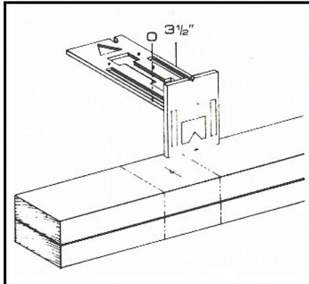
By marking at the points indicated, 2x8 corner walls are easily done.
