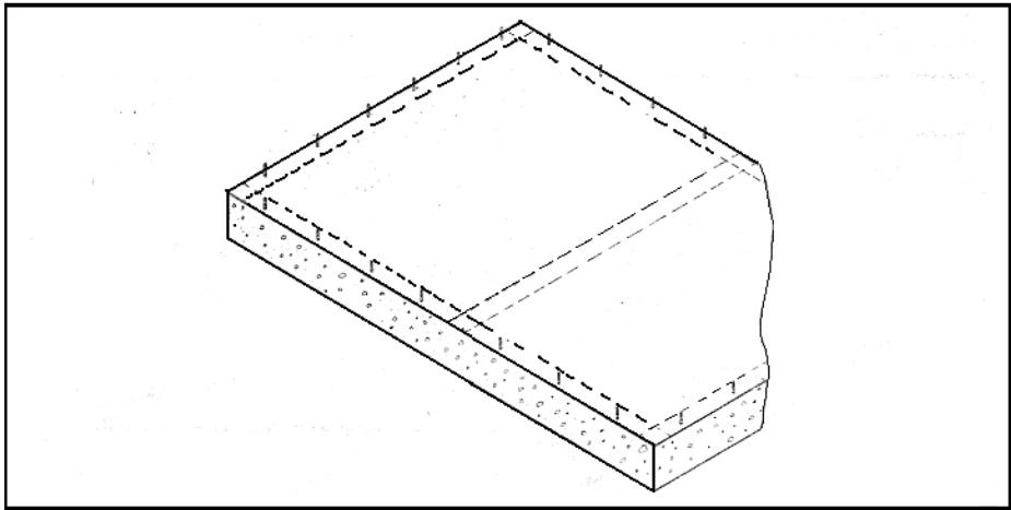
This illustration shows a finished chalkline layout on a concrete slab.
