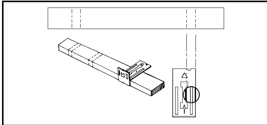
When marking stud locations the tool has a slot at 1 1/2 for double markings or (coupling in).
