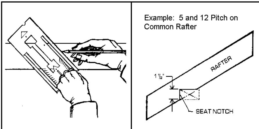
There are angle calibrations on one side of the blade, and hip, valley and common rafter calibrations on the other.
