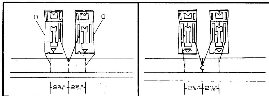
For 2x6 middle partition walls, line up the slot indicated, which is at  $2\frac{3}{4}$  with center line and mark along the edge of the tool, then duplicate the same procedure to the opposite side.
