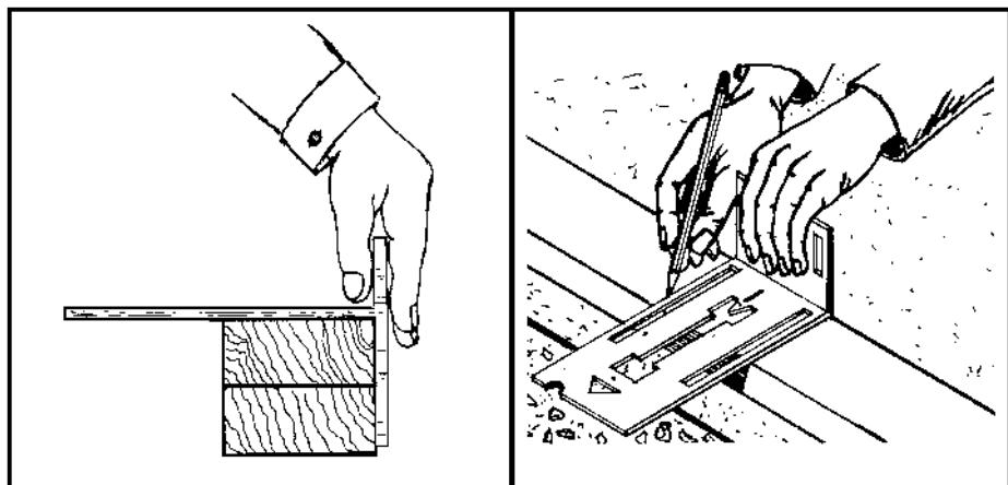
Shows the position in which the tool should be held and used.
