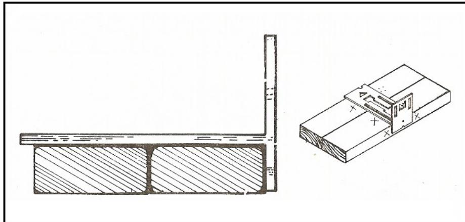
To mark wall stud locations on the sole and top plates, lay two, 2x4's in this position.
