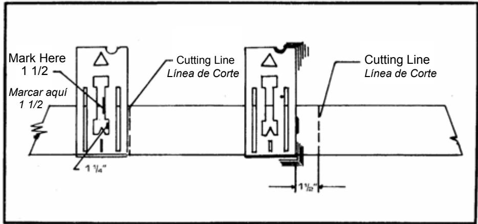
Hold tool with left hand and electric saw with right hand and cut on cutting line as shown.
