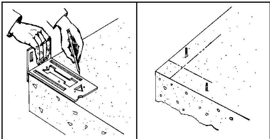
Outside and middle partition walls marked for snapping a chalkline without a tape measure.
