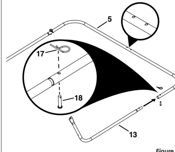
**STEP 8 (SEE FIGURE 8):** Install a rear hopper tube (5) onto the ends of the two upper hopper tubes (14). Secure them with two 1/4 x 1.11" clevis pins (18) and 3/32" hair pins (17).
