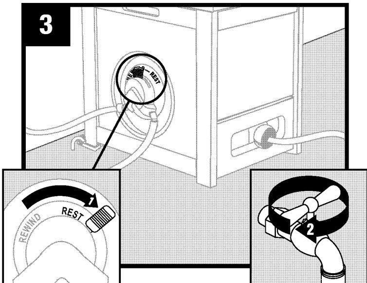
When finished rewinding garden hose, set the lever to REST and turn off the water source.
