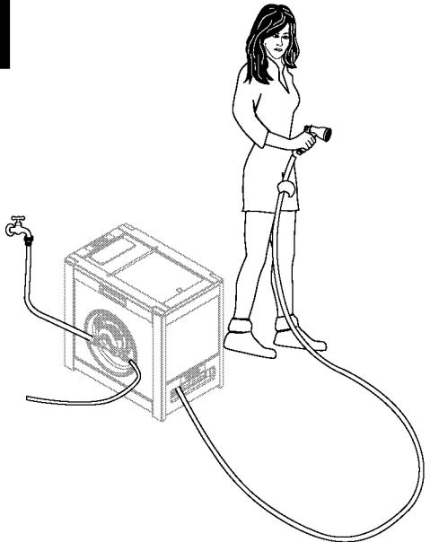
To wind your hose, pull the hose out away from your hose reel in a straight line. Then walk the end back to the hose reel so the hose is in a "U" shape in front of the reel. This assists in easier rewinding of the hose.
