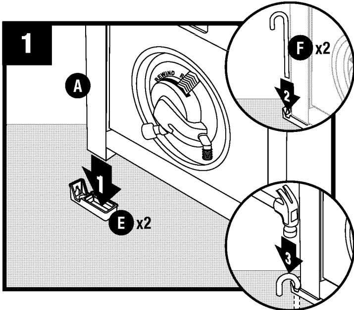
**Note:** Stabilizing your hose reel by staking is recommended.
