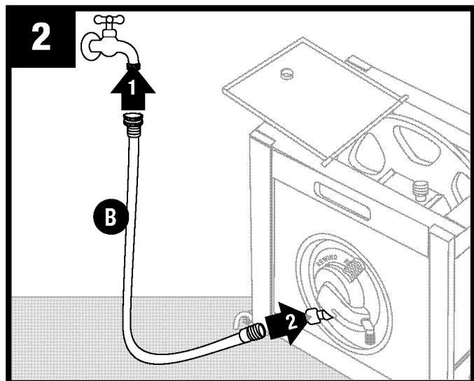
Connect Leader Hose (B). Thread male end of leader hose into in-tube. Thread female end of leader hose onto spigot.
