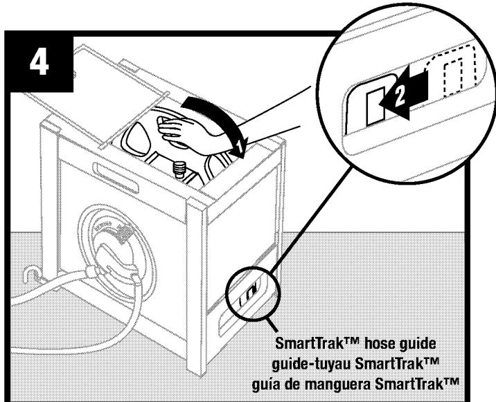
Manually rotate drum until the hose guide is in the left most position.
