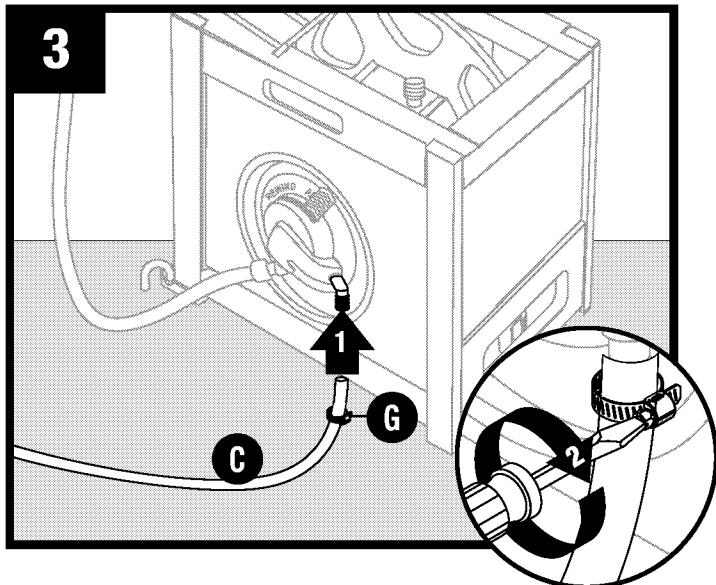
Connect drain hose (C) to the drain hose outlet. Secure with hose clamp (G). Place the opposite end in an area suitable for water drainage.
