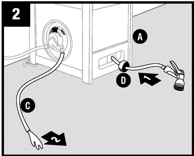
**During rewind, approximately 4-6 gallons of water will be discharged from the drain hose. Discharged water can be collected for use in watering plants or outdoor cleaning.**
