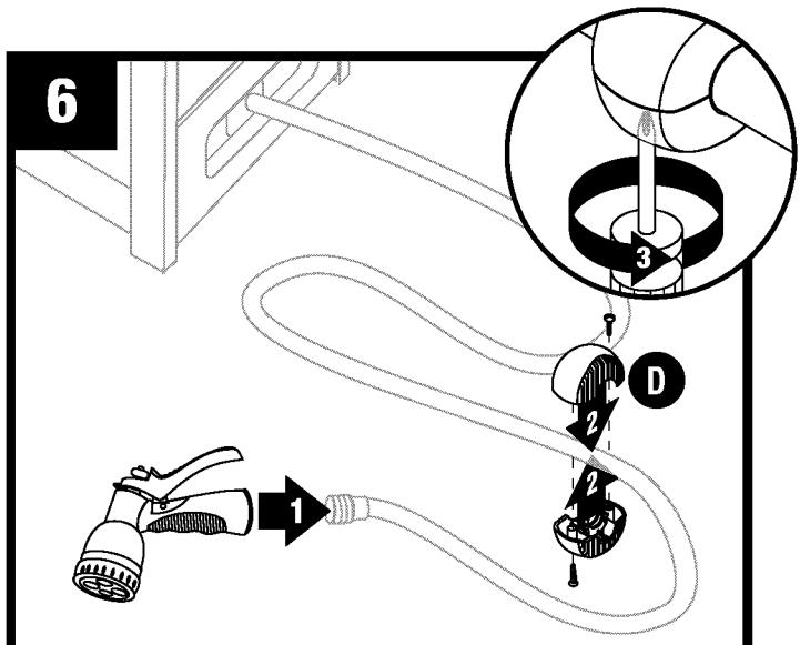
**Connect The Garden Hose.** If hose has a rigid sleeve, slide hose sleeve to the other end of the hose.
