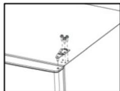
3. Remove the protective covers with a Phillips screwdriver through the back side, and save the protective covers.
