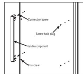
1. Use allen wrench to loose the fix screw and take out the handle component.
