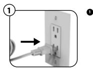
Plug Power Cord into a polarized outlet.
