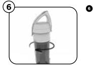
Replace the Dustbin Cover Assembly and twist clockwise to secure to the dustbin.
