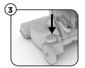
Tap the Vacuum Tilt release pedal ß to unlock the vacuum from the upright position.
