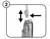
Insert the handle post into the top of the vacuum. Ensure the screw hole is facing toward the front of the vacuum.
