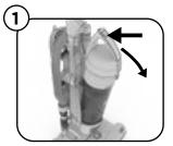
Press the Dustbin Canister Release and pull out to release.
