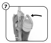
Attach Dustbin Canister onto the vacuum and push back until the Canister Release clicks into place as shown below.
