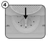
Height Adjustment: Adjustable height control allows you to change the height of the floor brush depending on your floor type. When vacuuming on thick carpet, adjust toward the Tall Carpet setting. For thinner carpet and hard floor, adjust toward the Hard Floor setting. Use the adjustment to satisfy your ideal vacuuming performance.
