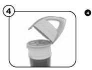
Lift the Filter Housing Release to gain access to the HEPA and foam filters. Remove the HEPA and foam filter, tap to dislodge fine dust and then rinse under cold water as needed for a deeper clean **Allow to FULLY dry (24hrs recommended) before re-assembling.**
