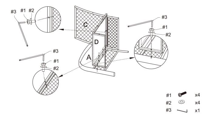
Step 3. Attach right arm panel (part B) to back panel (part C) and seat panel (part D) using bolts (part #1), washers (part #2) and allen wrench (part #3).
