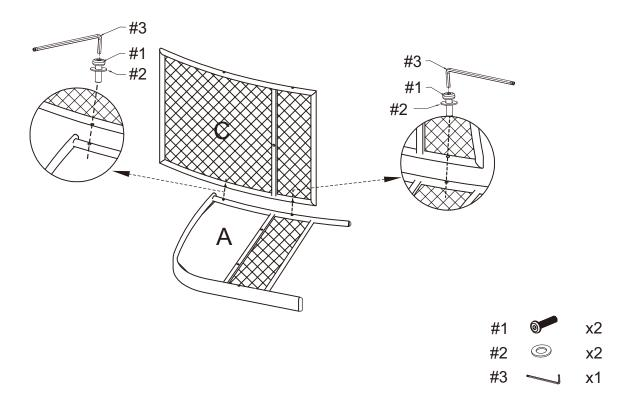
Step 2. Attach seat panel (part D) to left arm panel (part A) and back panel (part C) using bolts (part #1), washers (part #2) and allen wrench (part #3).
