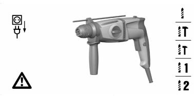
Set the function selector switch to the "Drilling"
