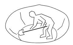
step 3: Begin digging always remembering to stay inside of your outline. Allow for plant ledges and basic shape of your pond. Level the edge of your pond by using a carpenter's level on straight 2 x 4 placed across your pond. This will show if one side needs to be adjusted. Repeat this process for the width and length of your pond until the perimeter is completely
