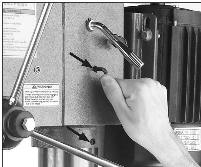
Figure 22. Securing headstock to column.
