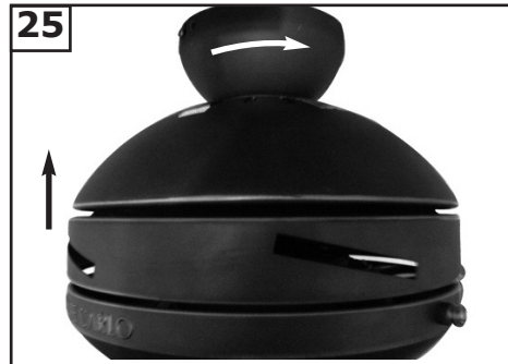
25 Lift fan to mounting bracket, aligning the "L" shape holes with the screws on the mounting bracket. Turn the fan clockwise to lock in position. Install the other 2 screws included in hardware bag and tighten all 4 securely.
