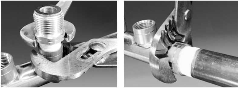
Figure 4.3 Supporting Manifold When Attaching Fittings
