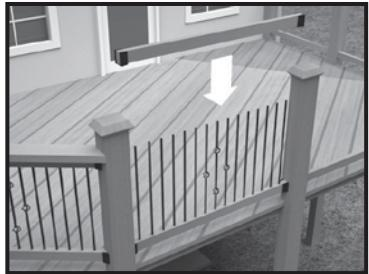
**6.** Once all balusters are set over bottom rail EZ Mounts or into RP Shoes, set the top rail by appropriately aligning the balusters and top rail EZ Mounts or RP Shoes. Attach top rail to support posts on each end using Fortress Rail Bracket (sold separately).
