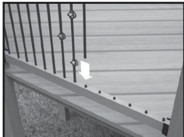
**5.** Set each baluster over bottom rail EZ Mounts or into RP Shoes per your design choice of plain balusters and/or basket balusters.
