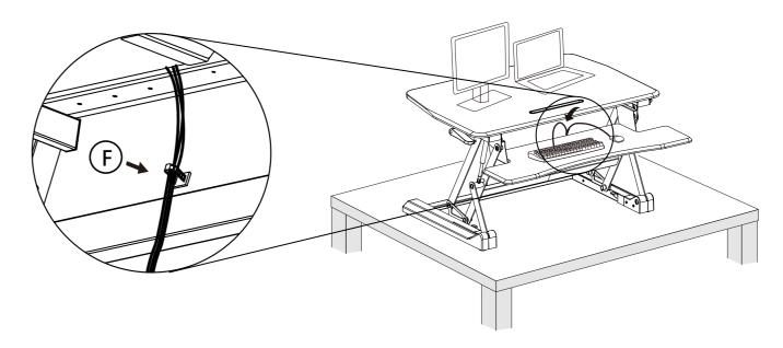
Stick the WIRE CLIP (F) to back of the crossbar. Use this clip to route cables from keyboards, mice and monitors through the <u>REAR</u> of the desk.
