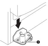
2 Fit the hinge 2 over the hinge lever latch 3 and slot it into place. Rotate the lever 4 clockwise and fasten the hinge.
