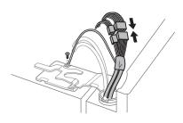
Push the water supply lines into the hole on the top case and pull them through the backplate.
