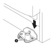
Fit the hinge 2 over the hinge lever latch 3 and slot it into place. Rotate the lever 4 counterclockwise to secure the hinge.
