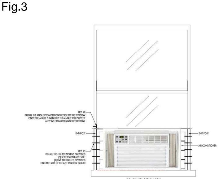
ELEVATION VIEW OF THE WINDOW WITH THE A/C WINDOW GUARD IN PLACE
