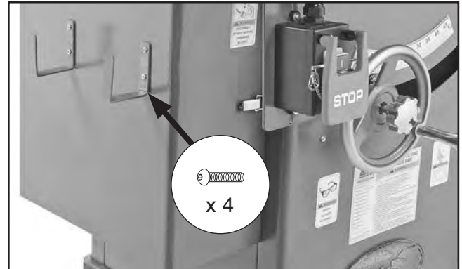
Figure 20. Fence resting brackets installed.
