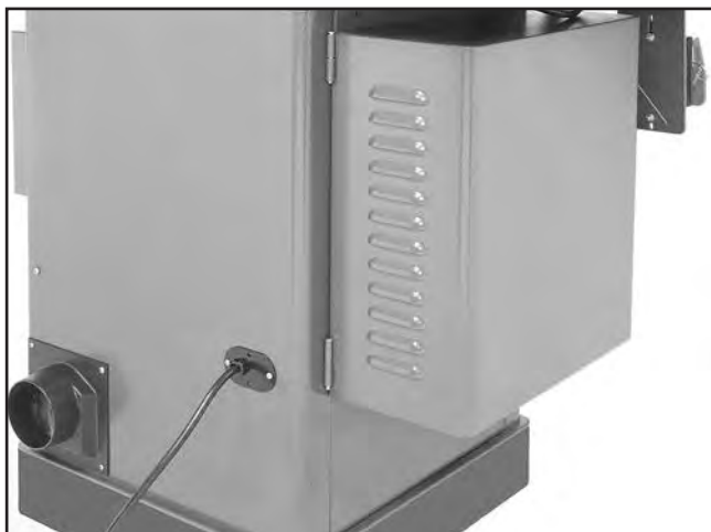
Figure 19. Motor cover installed.
