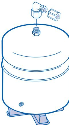
Adjust air pressure in the tank to between 5 and 7 psi. You will need an accurate digital air pressure gauge.
