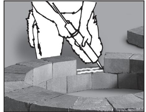
**6.** Once the 2nd course is all lined up, carefully remove one block at a time and apply two thick beads of concrete adhesive to the center of the blocks. Reinstall the block and push down firmly. Continue for all remaining blocks on 2nd course.
