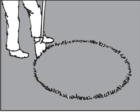
**1.** If putting your fire pit on a lawn, mark a 53-inch diameter circle and remove all sod and roots inside the circle. Dig approximately 2 inches deep. If putting your fire pit on a patio, mark the circle with chalk and skip ahead to step 4.
