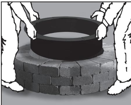
**8.** Next, lower the fire pit liner inside the blocks. The outside flange of the liner should be centered and rest on the inside edge of wall block units.
