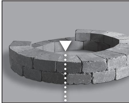
**5.** After the 1st course is set and leveled, start the 2nd course by placing the center of the top block in alignment with the joint between the blocks below. Continue this all the way around the circle.
