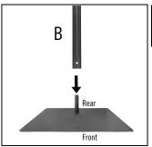
Place the base on the floor, with vertical upright closest to the base's rear. Insert the bottom of tube B into the base upright and secure with a nut and bolt provided. Tighten with wrenches until bolt engages nylon lock on nut.
