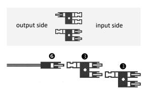
With the other 15-ft MC4 cable **⑤**, connect one branch connector **⑤** with the "male" output to the "female" end of the cable. Connect an additional "male" output branch connector **⑤** to the attached branch connector.
