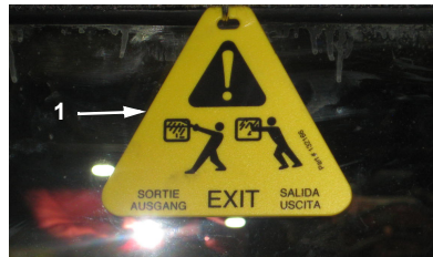
Figure 3 Rear Window Emergency Exit
