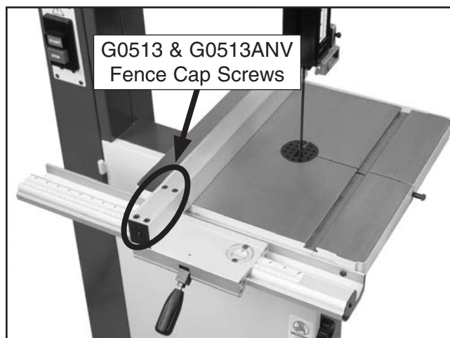
Figure 58. G0513 & G0513ANV fence caps screws.
