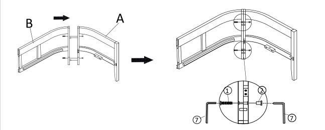
Place the Right Leg Panel (B) upright as shown in the picture above onto a clean, soft surface to avoid any scratches or damage to the product.
