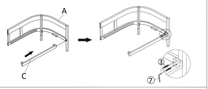
With assistance from your adult partner(s), attach the Support Bar (C) to the assembled parts in Step 2 by using Bolts (③) and the Allen Wrench (⑦) as shown above. **DO NOT** fully tighten the Bolts at this time.
