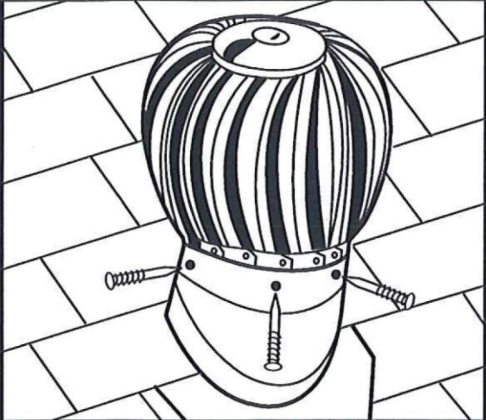
**Attach Turbine Head... Set turbine head firmly on the crimped base collar. Attach with three sheet metal screws (included) through holes in the turbine base ring.**
