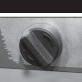
Fully open LP bottle valve. Turn valve to medium position. Allow gas to flow to burner. Immediately turn rotary ignitor. The ignitor should spark and light the burner. If ignition does not occur in 5 seconds, turn the burner control(s) off, wait 5 minutes, and repeat the lighting procedures.
