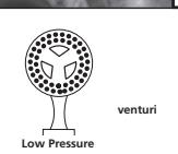
**Still Yellow:** Shut off valve(s) at stove and fuel tank. Through air shutter opening, clean venturi (burner neck) of obstructions such as cobwebs, dirt or bugs.
