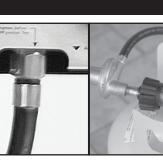
Attach regulator to tank. Check all connections to ensure tightness. With all valves in the off position, apply a soapy water solution to all fittings, valves and connections. Turn gas on at the tank and check for leaks at all connections. Small bubbles will appear if connection leaks. Tighten as needed.
