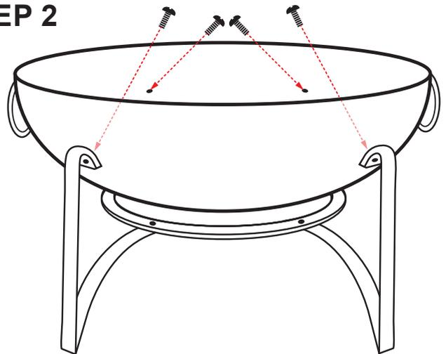
Align the holes in Fire Bowl (A) with the holes on the top of Legs (B). Hand-tighten 4x Bolts (G). Tighten all bolts with a Phillips screwdriver (not included).
