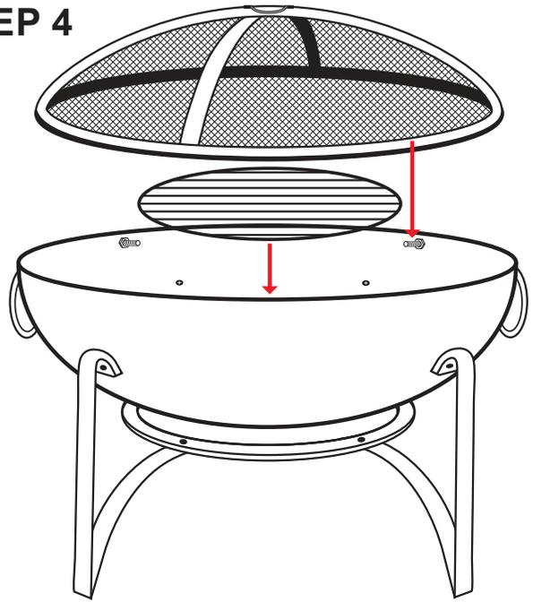
Place Log Grate (D) into Fire Bowl (A) and Spark Screen (E) onto Fire Bowl (A).
