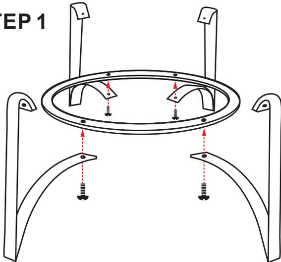
Align the holes on Legs (B) with the holes on Support Ring (C) and hand-tighten 4x Bolts (G).
