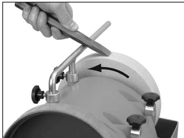
Figure 23. Example of properly grinding against wheel rotation.
