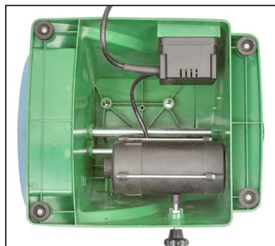
Figure 40. Motor and overall wiring.
