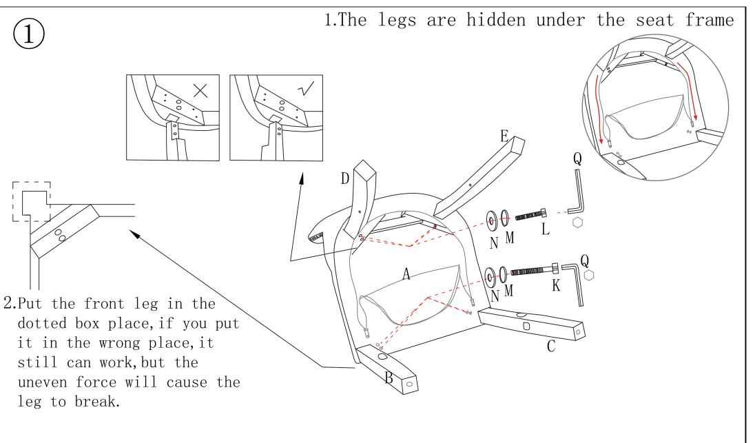
3. Tighten all the screws to 80% of maximum tightness
